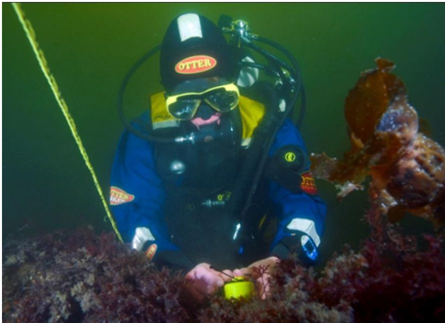
Figure 1: Diver attaching Aquatic-2 dataloggers to a weighted chain
